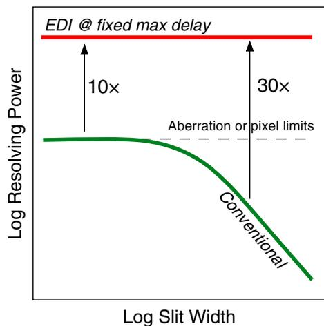
**Fig. 46** Notional diagram: the EDI surmounts classical limits to resolution from native spectrograph lens aberrations or detector pixel Nyquist sampling requirements. EDI resolution  $\text{Res} \sim \tau_{\text{max}}/\lambda$  is independent of slit width.
