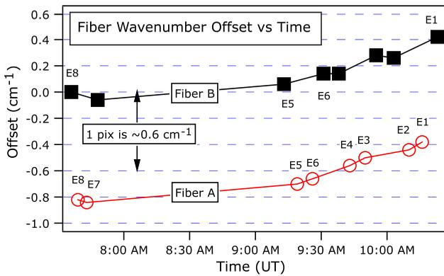
**Fig. 36** Bulk translation of the native spectrum along the dispersion axis due to thermomechanical or changing gravity vector, and due to slit slant acting on vertical separation of fibers A and B, for star HD219134 on September 19, 2010.
