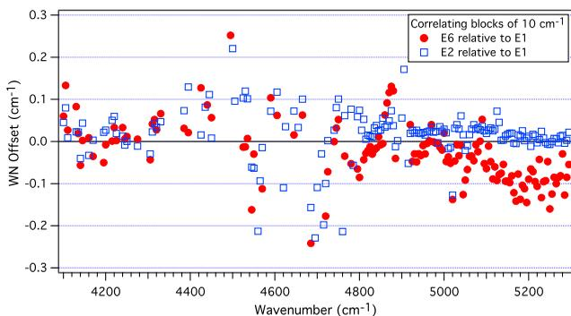
**Fig. 37** Irregular PSF drift of native spectrograph, versus wavenumber, correlated in  $10 \text{ cm}^{-1}$  chunks between E6 and E1 (red dots), and E2 and E1 (blue open squares), for the A-order and September 19, 2010, data of HD219134. The time-dependent bulk offset (Fig. 36) has already been removed.
