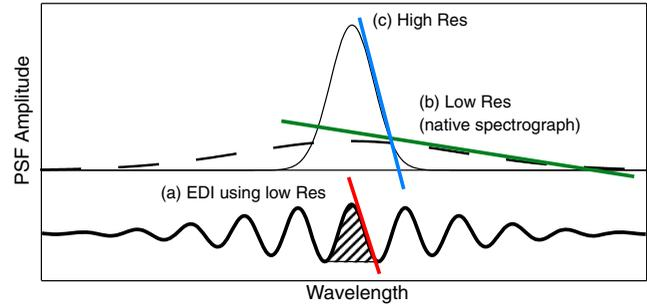
**Fig. 3** The EDI PSF (instrument response) is a corrugated peak (bold curve), which has a much higher slope (and thus higher Doppler sensitivity) than the low resolution native spectrograph alone (dashes). The slope of the sinusoid is proportional to the interferometer delay. For use in high-resolution spectroscopy, the subject of this report, the central area (cross-hatched) is made unambiguous by combining several wavelets of different periodicities (delays), as shown in Figs. 4 and 5.
