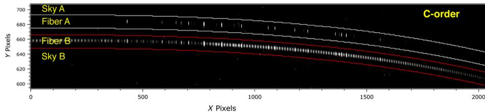
**Fig. 6** Example C-order of the 2-D echelle fringing spectrum covering 6700 to 8800  $\text{cm}^{-1}$  (left to right) over 2048 pixels. The three other orders (A, B, D) spanning 4100 to 11,000  $\text{cm}^{-1}$  (0.9 to 2.45  $\mu\text{m}$ ) are shown in Fig. 2 of Ref. 2. Fiber A (white curves) is ThAr lamp alone, fiber B (red curves) is Star + ThAr. Note the sinusoidal comb from the continuum. Data from 2010Sep19, #0756, star HD962, etalon E1 ( $\sim 0.1$  cm).
