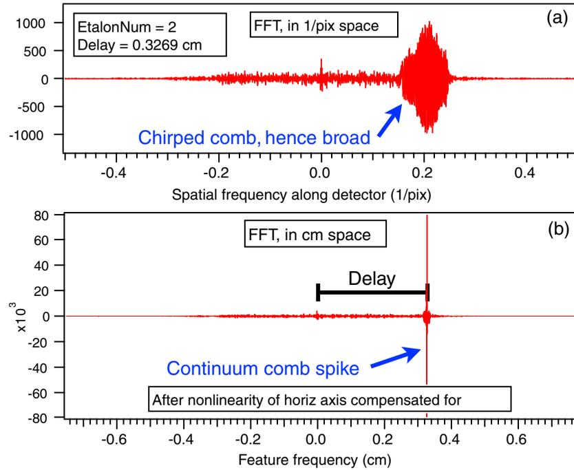
**Fig. 16** The effect of linearizing the horizontal axis from pixels to wavenumbers, and compensating for glass dispersion, is to narrow the comb spike. (a) The Fourier transform of whirl for delay E2 (0.33 cm) in 1/pixel frequency space, showing a broad continuum comb spike. (b) Linearized data, the spike is extremely narrow.
