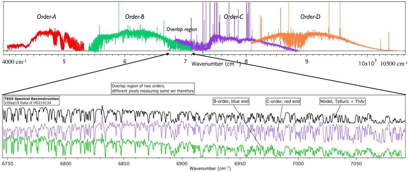
**Fig. 23** The TEDI reconstructed resolution boosted spectrum spans the four orders of TripleSpec spectrograph in NIR (4100 to 10,500  $\text{cm}^{-1}$ ), here observing HD219134 on September 19, 2010. The lower graph is zoomed in region of overlapping orders B and C, showing agreement between two very unrelated groups of pixels (on opposite sides of detector), and with telluric model<sup>19</sup> (black curve).
