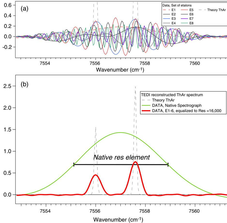
**Fig. 5** (a) Reconstruction of an otherwise unresolved ThAr doublet (7556, 7557.6  $\text{cm}^{-1}$ ) from many wavelets measured at multiple delays. (b) The native spectrograph (green curve) cannot resolve the doublet. The EDI reconstructed spectrum (red curve), which is sum of wavelets, then equalized to  $\text{RES} = 16,000$ , easily resolves the doublet.
