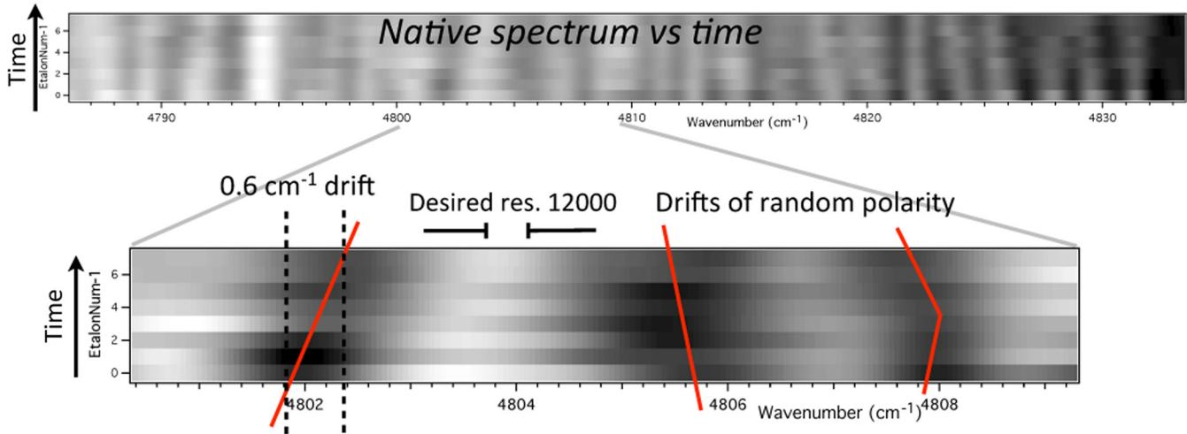
**Fig. 35** Large PSF irregularity in the native spectrograph to which EDI is robust. Row is native spectra of A-order versus etalon # (~10 min apart). The PSF shift  $\sim 0.6 \text{ cm}^{-1}$  versus etalon # is called “shear.” Bulk shear has already been removed here, and an irregularity remains. Note irregular change in shear polarity. Fortunately, for the EDI the native lineshape only affects the envelope of the wavelets, but not the internal shape.
