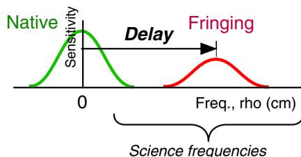
**Fig. 2** Heterodyning shifts the native spectrograph sensitivity peak from zero to a higher frequency where science frequencies typically reside, by amount equal to the interferometer delay  $\tau$ , and an amplitude 50%. Frequency in units of features per wavenumber ( $\text{cm}^{-1}$ ), conveniently has units of delay, units of cm.
