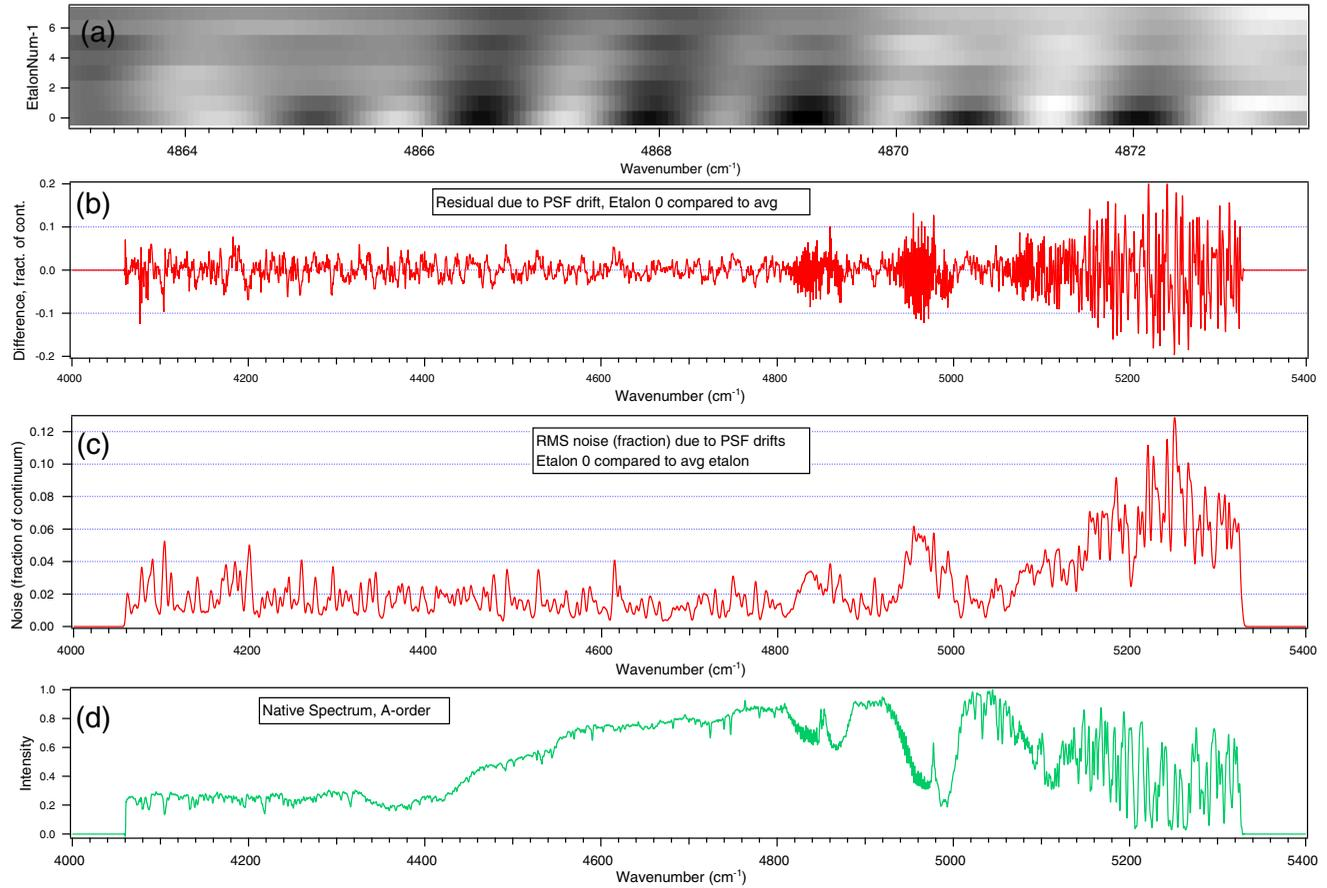
**Fig. 38** (c) Measured amount of (vertical) instrumental noise for A-order, as a fraction of continuum, due to (horizontal) PSF drift or width change, by subtracting the native spectrum averaged over all eight etalons (d) from each spectrum (a) measured individually for each etalon to produce about a 3% residual (b).
