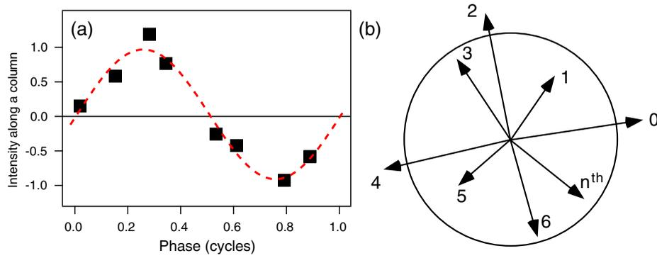
**Fig. 12** (a) Sine fitting is equivalent to a (b) vector construction where step phase and visibility are designated by vector length and angle, which can both be irregular. To isolate the nonfringing from fringing components the vector sum must be zero. The values of weights to achieve this are calculated from phase of ThAr features. Whatever arithmetic is performed on vectors is also performed on data.
