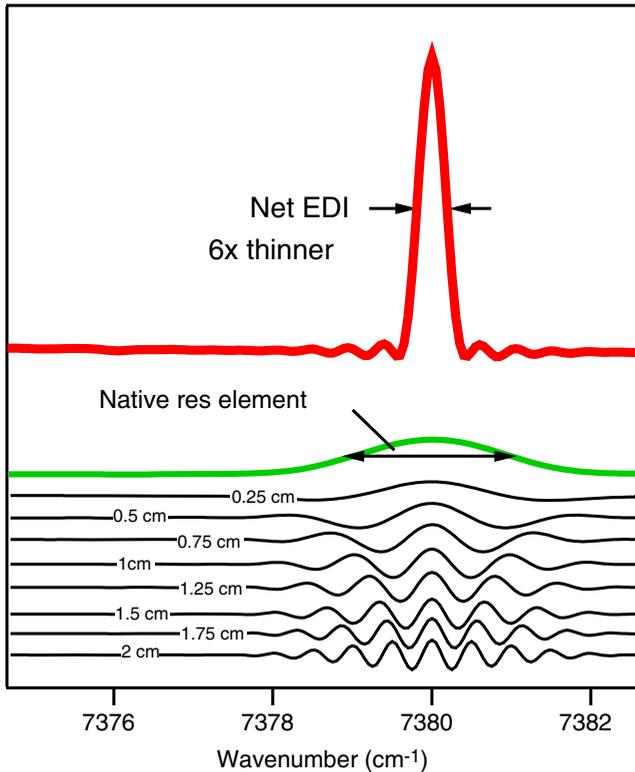
**Fig. 4** Simulated summation of several simulated wavelets, weighted in Gaussian equalization scheme, produces a single Gaussian PSF peak with minimal ringing (bold red) and thinner than the native spectrograph (green curve) by factors of several.
