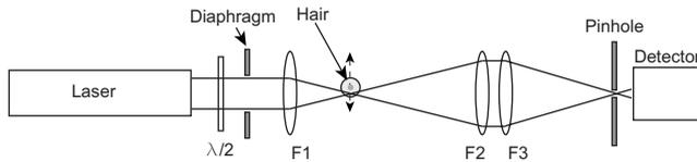
**Fig. 1** Schematic diagram of the confocal setup used for the measurement of collimated transmittance through a hair:  $\lambda/2$ , a multiorder half-lambda waveplate; F1, a  $20\times 0.4$  NA microscope objective; F2, a 40-mm-focal-distance lens; F3, a 100-mm-focal-distance lens.
