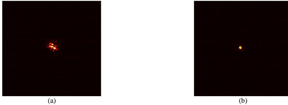
Figure 7 image of the focus camera (a) AO off and (b) AO on.
