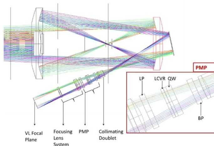
**Fig. 3** - Optical layout for the visible light path.
