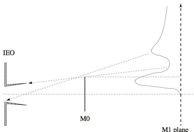
Fig. 6. - Sketch of the shape of the diffraction curve of IEO on the primary mirror.
