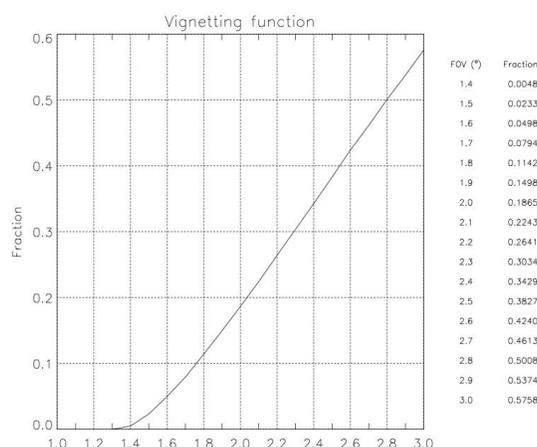
Fig. 2 - Vignetting function as a fraction of the entrance pupil defined by the IEO aperture as a function of the field angle.
