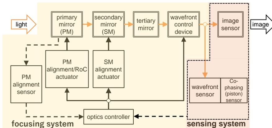
Figure 4. Block diagram of wavefront management system
