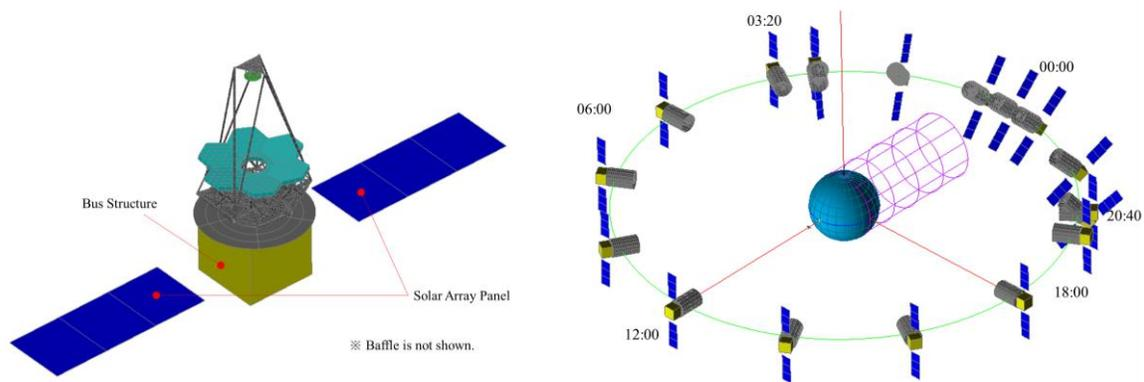
Figure 2. Thermal analysis model (left) and orbital configuration (right).
