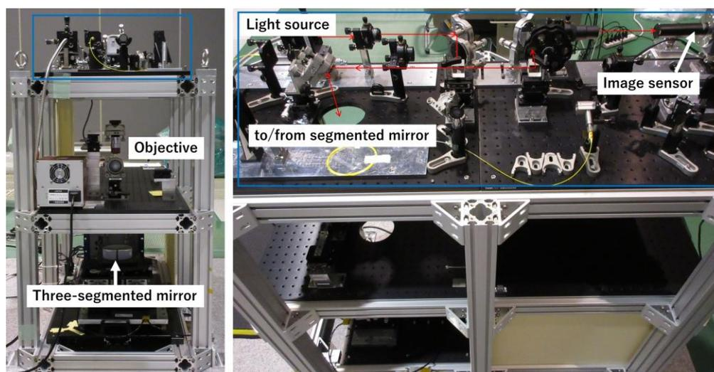
Figure 5. Miniature testbed for testing alignment procedure.
