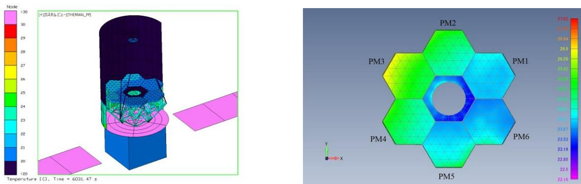
Figure 3. Temperature distribution of the satellite (left) and the primary mirror segments (right).
