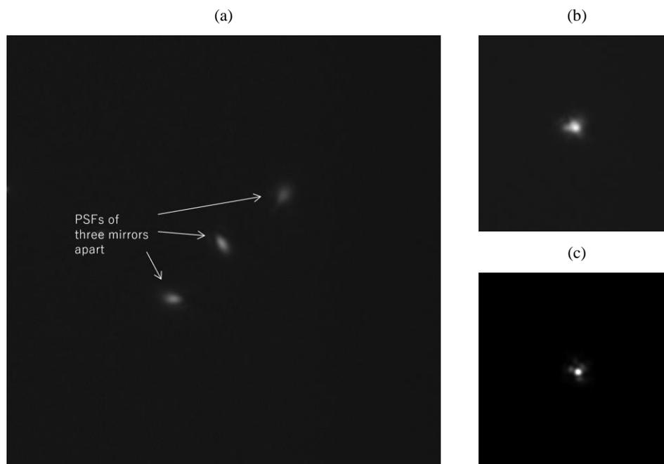
Figure 6. Obtained image before and after phasing. (a) unstacked three PSFs before tip-tilt adjustment (b) stacked and unsynthesized PSF (c) after completed PTT optimization
