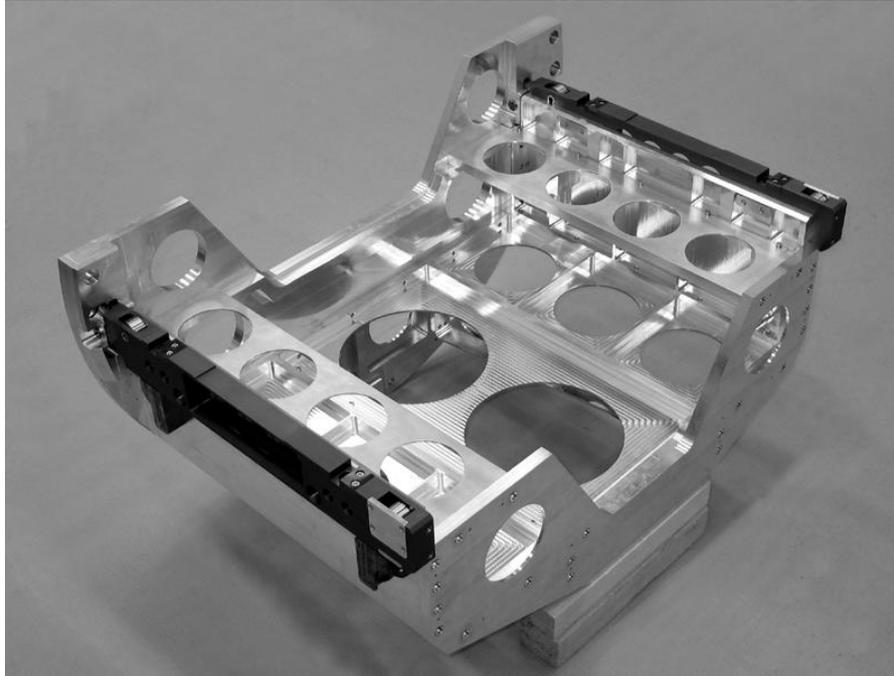
**Figure 7.** The fully assembled mounting structure of FIFI LS.
