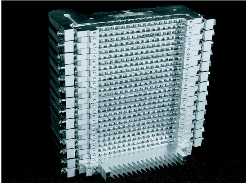
**Figure 12.** The 25 (+2 spares) stressed Ge:Ga detector modules of FIFI LS. the lower two modules are equipped with light cones.
