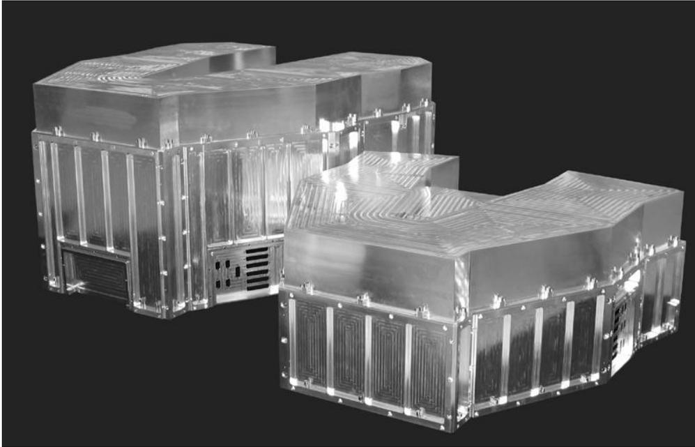
**Figure 9.** The radiation shields. The inner shield of the liquid helium system is in front and the outer shield of the liquid nitrogen system is in the background. Both shields will be covered with superinsulation on the outside and infrared black paint on the inside.
