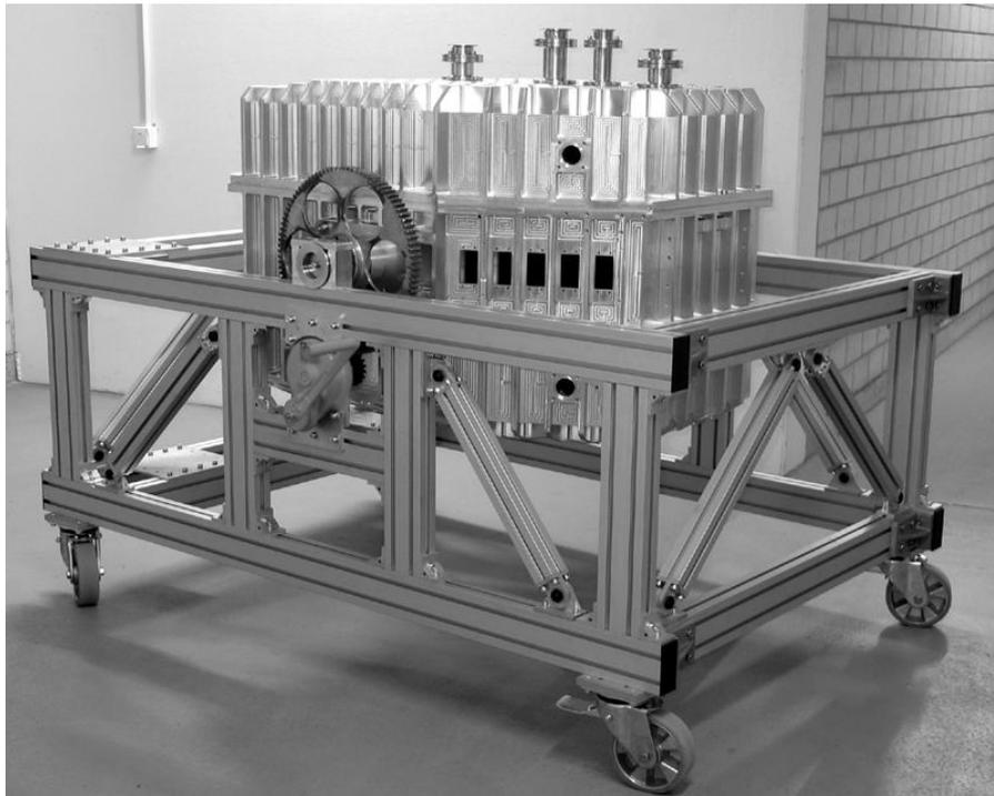
**Figure 6.** The FIFI LS vacuum vessel mounted on the instrument integration cart. The dimensions of the instrument are roughly 1 m × 1 m × 1 m.
