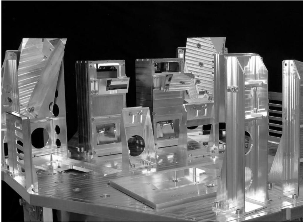
**Figure 10.** The FIFI LS optical system. Dichroic beam splitters, diffraction gratings and detector arrays are not installed. Compared to Fig. 4 the picture is upside down.
