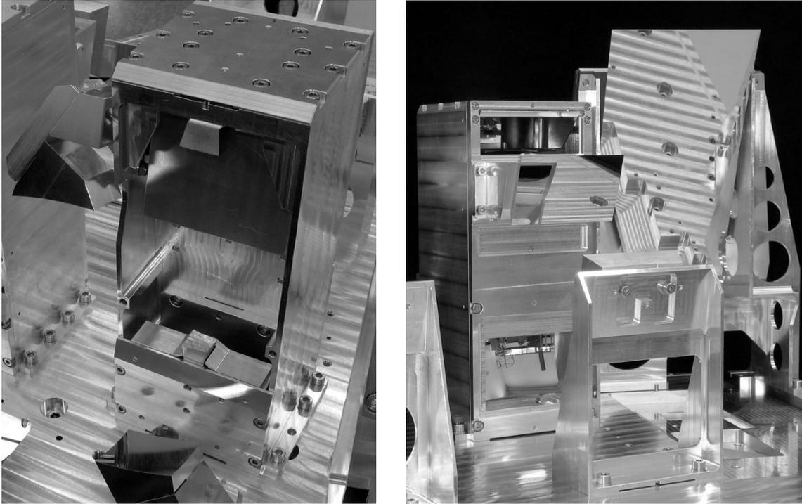
**Figure 11.** Details of the FIFI LS optics. The left panel shows the image slicer console and two of the magnification mirrors of the blue spectrometer. In the right panel a collimator mirror together with the imaging mirrors at the exit of the spectrometer and the image slicer console of the red is shown.
