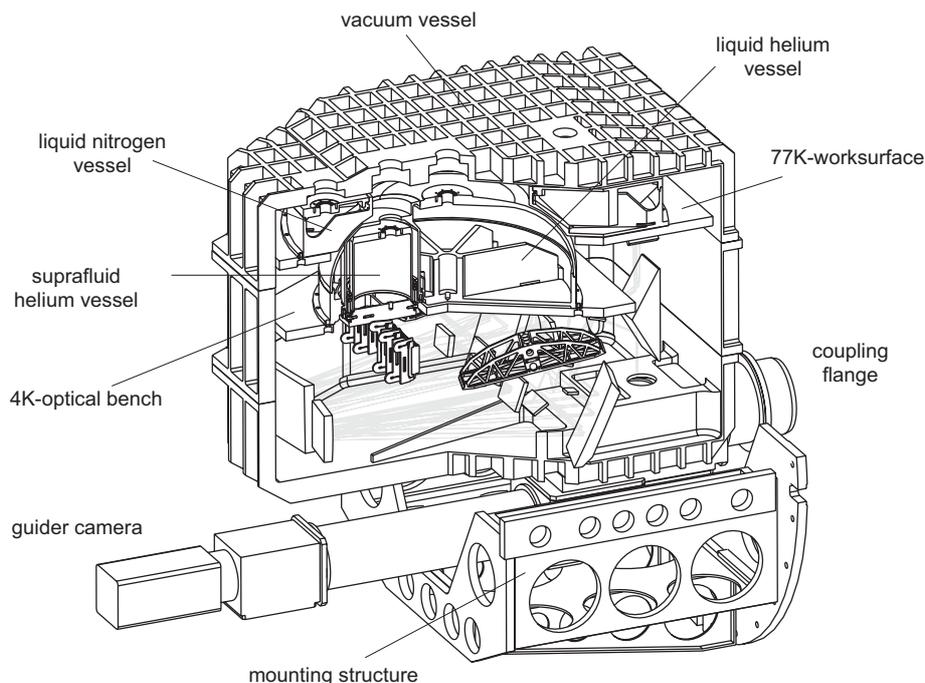
**Figure 1.** A cut through the FIFI LS cryostat. The optical components are mounted on the cryogenic plates. Light from the SOFIA telescope is entering the instrument from the right via the coupling flange.
