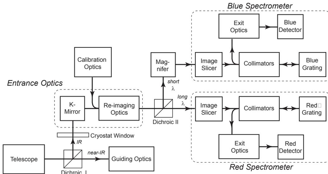
**Figure 3.** A block diagram of the FIFI LS optics. Calibration optics used to provide flat-fielding of the detector pixels can be switched into the path via a flip-mirror.
