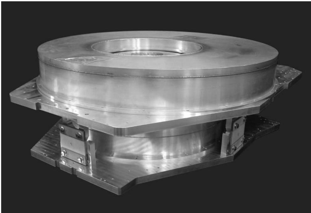
**Figure 8.** The preliminary assembly of the instruments cryogenic system. The assembly includes: the cryogen vessels, the cold worksurfaces (77K and 4K), and the G-10 and carbon fiber stand offs.
