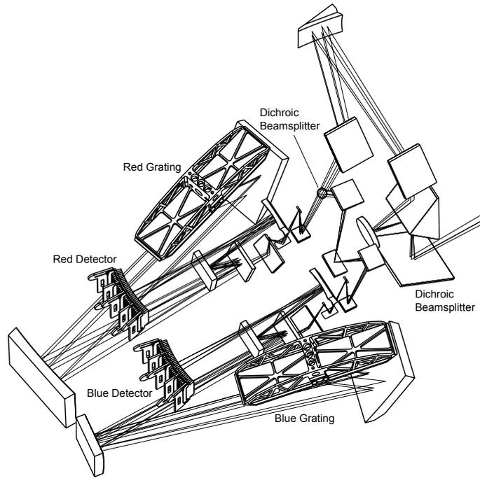
**Figure 4.** The optical system of FIFI LS. Light from the telescope enters at the right (close to 'Dichroic Beamsplitter').
