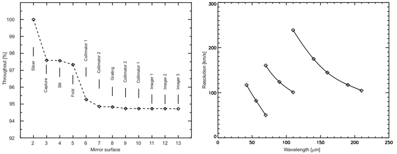
**Figure 5.** Left: The light loss through the optics due to diffraction and vignetting effects. Right: The simulated spectral resolution of FIFI LS.
