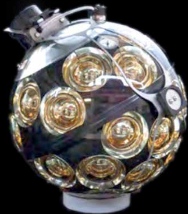
Photograph of a digital optical module (DOM), which houses 31 photomultiplier tubes plus the front-end and readout circuitry.
