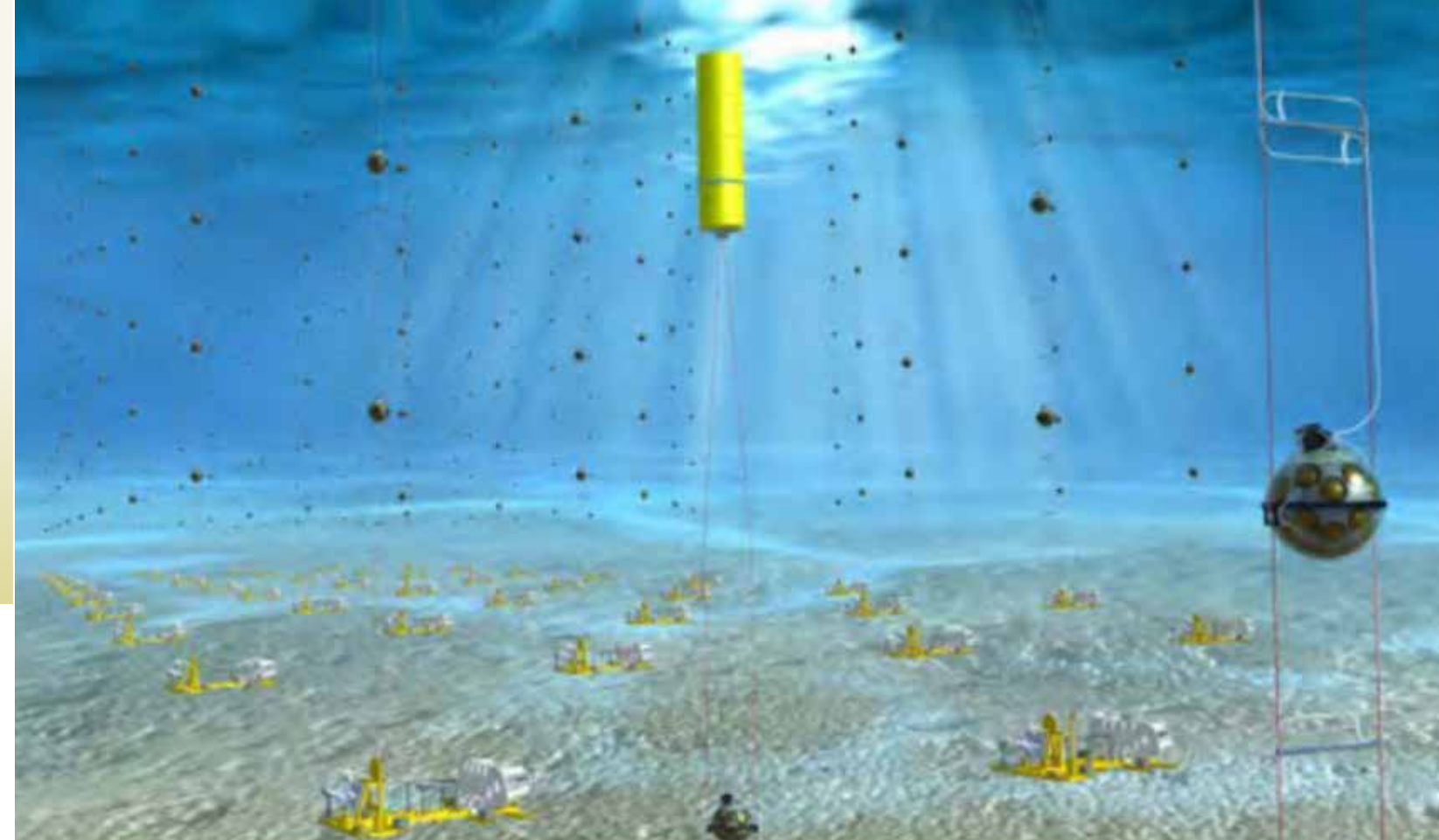
Artist’s representation of a deep-sea neutrino telescope, showing DOMs deployed in a 3D grid. Figures credit: Sebastiano Aiello et al., doi 10.1117/1.JATIS.7.1.016001
