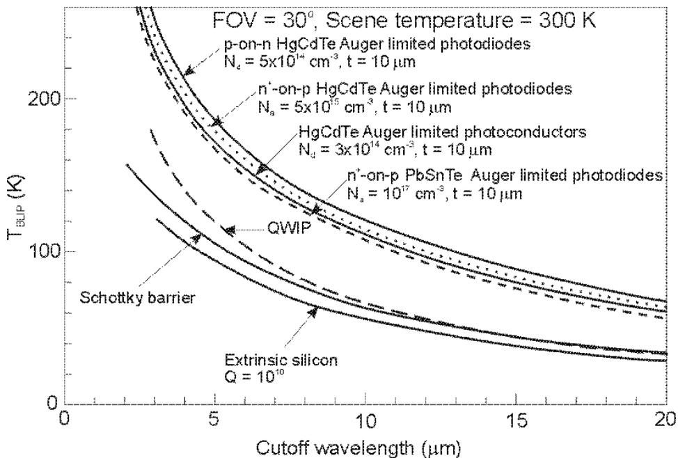
Fig. 2. Estimation of the temperature required for background limited operation of different types of photon detectors. In the calculations  $\text{FOV} = 30^\circ$  and  $T_b = 300\text{ K}$  are assumed (after Ref. 6).
