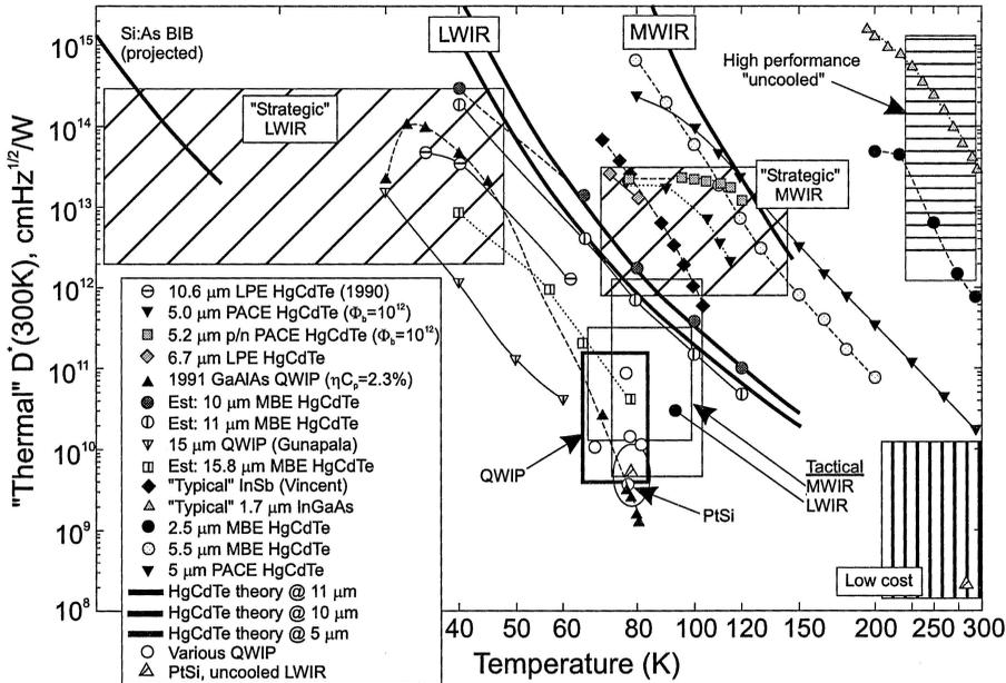
Fig. 1. Thermal  $D^*$  versus operating temperature for different FPA technologies (after Ref. 1).
