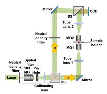
Fig. 1 The bitelecentric DHM in transmission configuration, including MO, beamsplitters (BS), object beam (O), reference beam (R), and CMOS camera.
