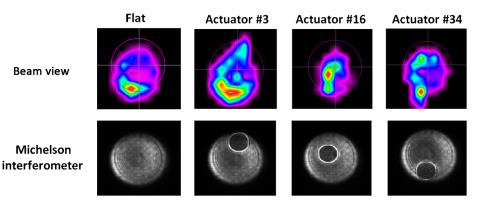
Fig. 7 Example results looking at different actuator "pokes" on the MEMS DM. The "beam view" is the laser intensity as reflected off of the MEMS DM.
