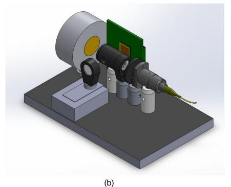
**Fig. 3** (a) Top view of the Michelson interferometer payload that fits into a 95 mm  $\times$  150 mm footprint, which will fit in the 3U CubeSat payload volume. (b) Isometric view of the Michelson interferometer payload. A diode laser passes through a pinhole and is collimated before entering a 50/50 nonpolarizing beamsplitter. Light is reflected off both the flat mirror and the DM and is combined on the detector to form fringes.
