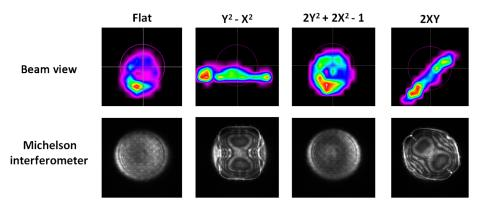
Fig. 8 Example results looking at different Zernike polynomials on the MEMS DM. The "beam view" is the laser intensity as reflected off of the MEMS DM.
