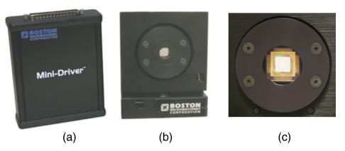
**Fig. 2** Boston Micromachines Mini  $6 \times 6$  (32 actuator) deformable mirror (DM) and drive electronics (Ref. 50). (a) Driver board packaging that would be removed; (b) mirror in packaging of which the exterior would be removed; and (c) close-up of the mirror. The drive electronics board could fit in a CubeSat without the packaging and with some minor modifications to the board.
