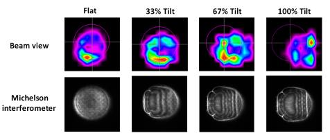
Fig. 6 Example results looking at different steepness tilts on the MEMS DM the Michelson interferometer prototype (Michelson without nanopositioning stage here). The "beam view" is the laser intensity as reflected off of the MEMS DM.
