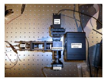
**Fig. 4** CubeSat-sized MEMS DM Michelson interferometer prototype experiment. The setup includes a 1.5  $\mu$ m stroke Boston Micromachines Mini DM, a Thorlabs CPS180 635 nm 1 mW round beam collimated laser diode module, a cube beam splitter, a pinhole spatial filter, a neutral density filter, a flat mirror, and a Thorlabs DCC1545M ½ in. monochrome CMOS camera. A MATLAB interface to the mirror driver is commanding the 32 actuators into a "tilt" or "tip."
