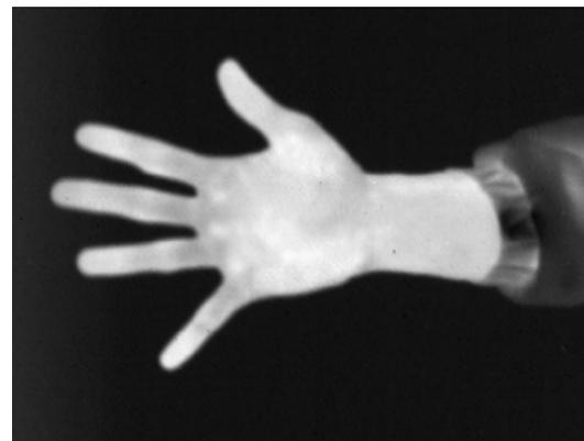
**Fig. 15** Thermal image obtained by QVGA type IRFPA (HX0830) with the new structure pixel of  $23.5\ \mu\text{m}$  pitch (with  $F/1$  at 60 Hz).
