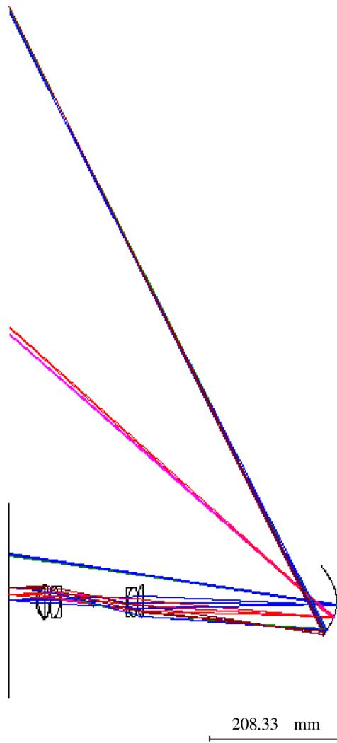
**Fig. 8** The LCoS image is formed on the screen through the refractive lens and reflective mirror.
