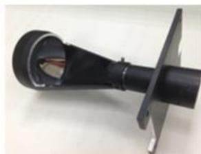
Fig. 19 Utmost Co. LCoS projection engine with self-designed optics and optomechatronic mount.
