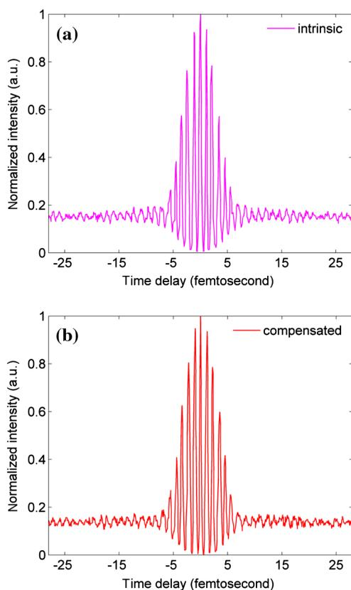
**Fig. 2** Interferometric autocorrelation trace of (a) intrinsic sub-10 fs mode-locked pulse from the untuned laser agrees well with that of (b) GDD-compensated sub-10 fs TLP in situ.
