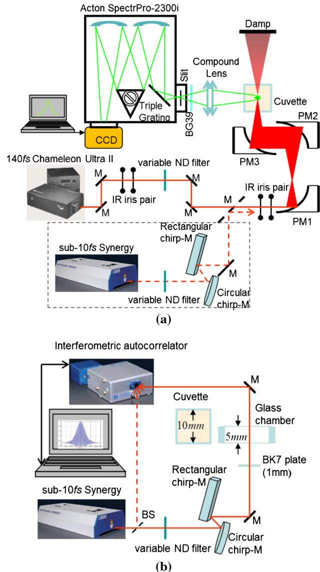
**Fig. 1** (a) Experimental configuration for TPEF measurements: PM (parabolic-mirror), ND (neutral density) filter and (b) experimental set up for testing the optimal GDD compensation.
