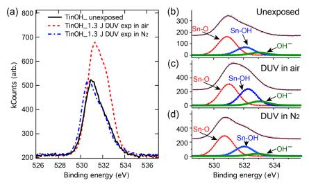
Fig. 4 The O 1s core-level spectra for TinOH unexposed sample, sample exposed in air, and sample exposed in  $N_2$ . (a) Core-level spectra sharing the same scale on the ordinate axis. (b)–(d) Least squares fits for each sample using the three-component model described in the text.
