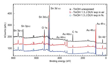
Fig. 2 Overview HAXPES spectrum of TinOH unexposed sample, TinOH DUV-exposed in air, and TinOH DUV-exposed in N<sub>2</sub>. (The spectra are displaced vertically to avoid overlapping of the peaks).
