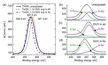
**Fig. 3** Sn  $3d_{5/2}$  core-level spectra for TinOH unexposed sample, TinOH DUV-exposed in air, and TinOH DUV-exposed in  $N_2$ . (a) Core-level spectra sharing the same scale on the ordinate axis. (b)–(d) Fits for each sample using the two-component model described in the text.
