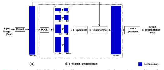
**Fig. 6** An overview of PSPNet. The size of feature map channels is denoted below each box. The size of the last feature map in (a) is 1/8 of the input image size.
