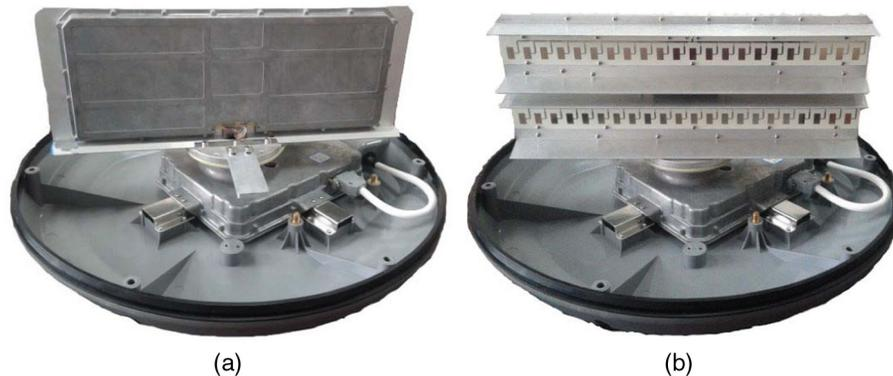
**Fig. 8** The scanning radar system [(a) front side and (b) back side] utilized to collected scattering data.
