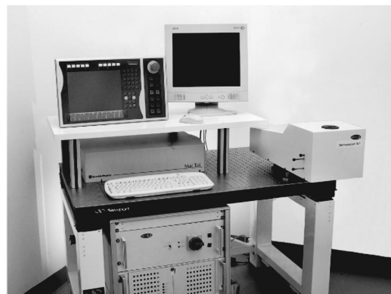
Fig. 1 Photograph of the multiphoton imaging tool DermalInspect 110 for 4-D autofluorescence and SHG imaging with intracellular spatial resolution and 250-ps temporal resolution.
