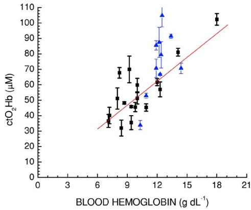
**Fig. 3** Absolute comparison between invasively measured hemoglobin and DOS measured  $ctO_2Hb$ . Nontransfused as well as transfusion infants are shown (squares). Error bars represent the SD of the results from repeated individual measurements (17 subjects, 34 measurements). The solid line is an error-weighted ( $r=0.83, p<0.0001$ ) fit involving the initial measurements on all 17 subjects. Squares represent the post-transfusion measurements (but were not included in the fit).
