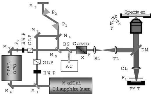
**Fig. 1** Schematic of the experimental setup. HWP: half-wave plate; GLP: Glan-laser polarizer; M: mirror (M1 and M5 mirrors held in flip mounts); BS: beam sampler; P: prism; AC: autocorrelator/spectrometer; SL: scanning lens; TL: tube lens; DM: dichroic mirror; CL: collection lens; F: filter; and PMT: photomultiplier tube.
