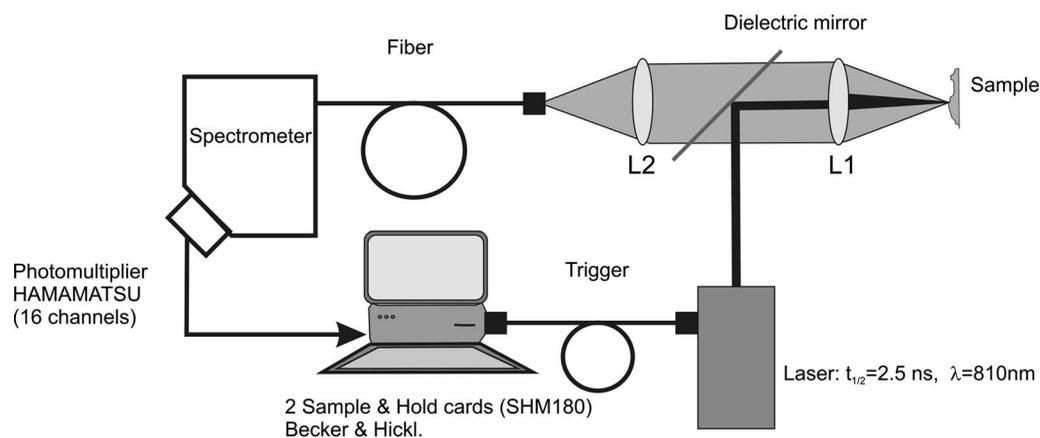
**Fig. 2** Scheme of the fluorescence measuring device LIMES 16-P (for details, see text).
