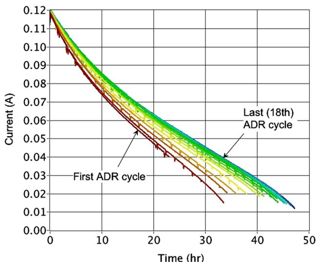
**Fig. 5** Demagnetization curves for stage 1 for the 18 cycles completed on orbit. Time is from the first crossing of 50 mK after recycling. The exponential approach of the helium tank to its steady-state temperature gave rise to a gradual increase in hold time with each cycle.
