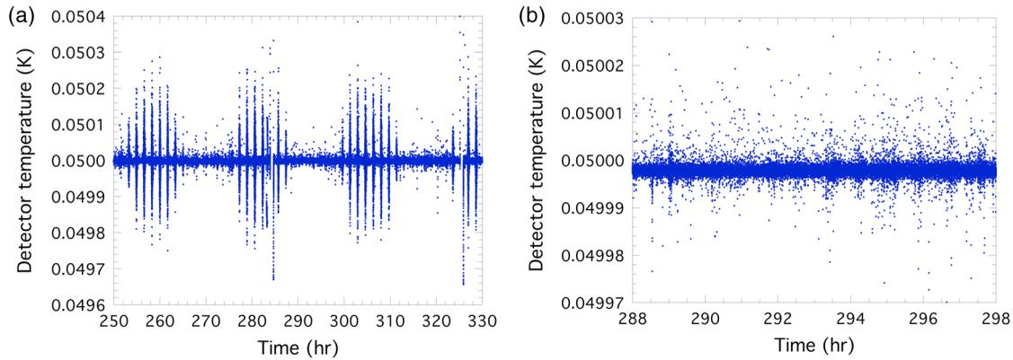
**Fig. 6** Detector array temperature (a) showing the effect of high-energy particles during passes through the SAA, and (b) when Hitomi was outside the region of the SAA.
