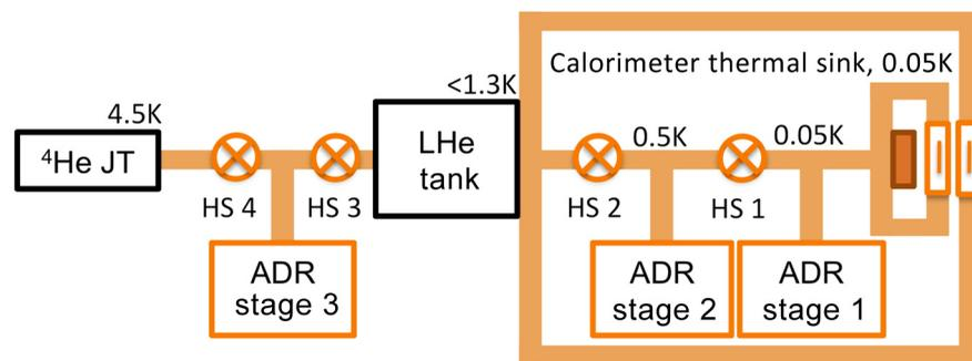
**Fig. 1** Thermal schematic of the subset of the Hitomi cryogenic consisting of the ADR, helium tank, and JT cryocooler.
