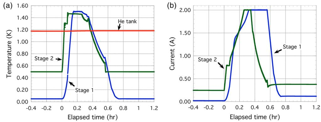
**Fig. 3** (a) Temperatures and (b) magnet currents during an ADR recycle (ground test data).
