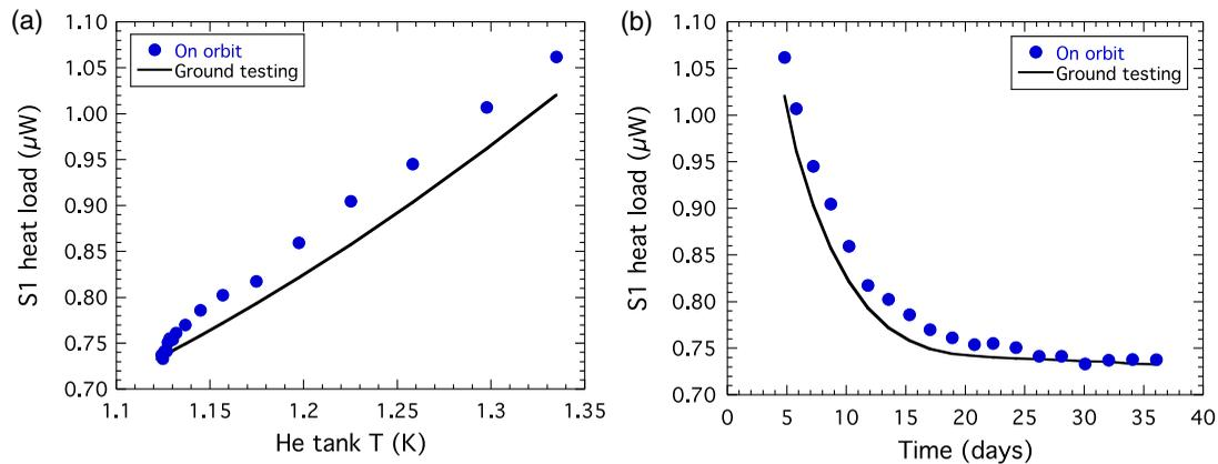
**Fig. 7** Heat load on stage 1 for each ADR cycle on orbit as a function of (a) helium tank temperature and of (b) time on orbit. The solid lines indicate the expected heat loads at the indicated tank temperature or time based on ground testing.
