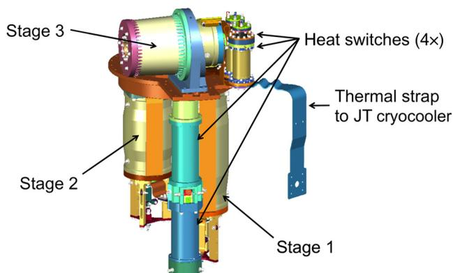
**Fig. 2** Solid model representation of the SXS three-stage ADR.
