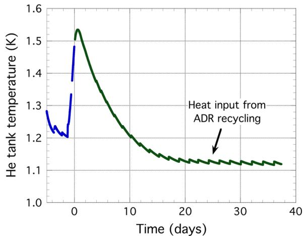
**Fig. 8** Helium tank temperature from shortly before launch through to the end of operations on day 38. The increase leading up to launch was due to closure of the vent valve and periodically turning off the cryocoolers.
