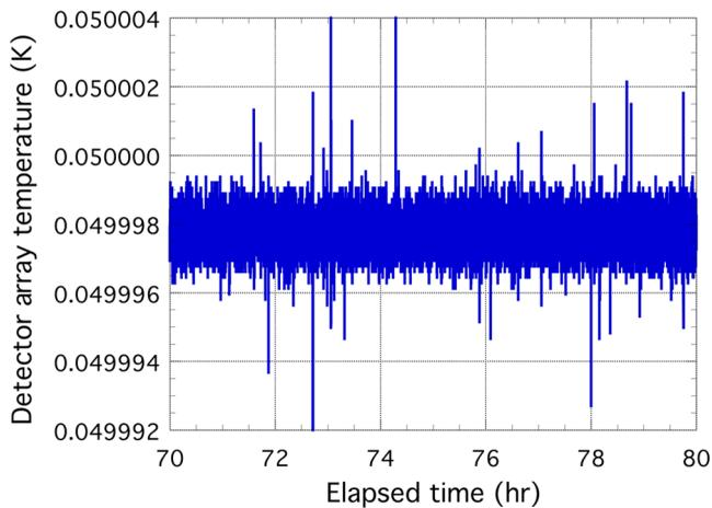
**Fig. 4** Typical detector array temperature during ground testing at 50 mK.
