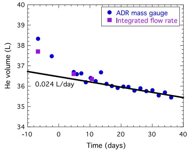
**Fig. 9** Helium volume as determined from ADR recycles, compared with a direct measurement after the final top-off that was then integrated to reflect boiloff loss as the helium cooled. The solid line represents a loss rate of 0.024 L/day.
