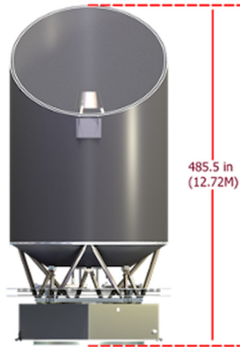
Fig. 7 Origins observatory dimensions (front).
