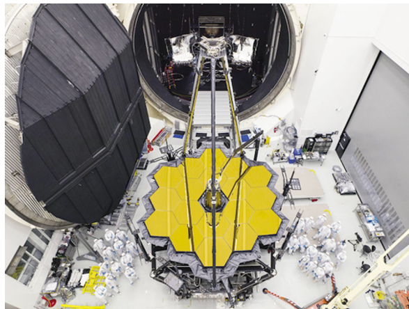
Fig. 14 JSC chamber A supports Origins “test as you fly.” The JWST OTIS is shown rolling into the JSC chamber A. Chamber A and its helium cooled shroud provides a perfect environment for thermal verification of Origins with and without the spacecraft.
