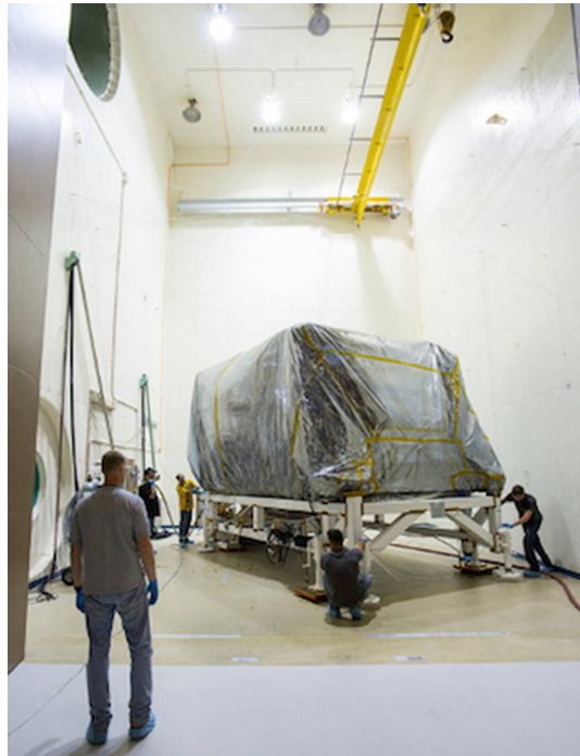
Fig. 13 The GSFC acoustic chamber can easily accommodate testing the Origins CPM. Note that this chamber is not large enough for the fully assembled Origins observatory. This test will be performed at the JSC or another suitable facility.
