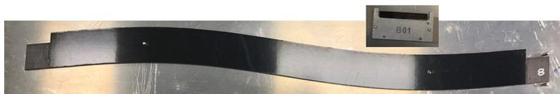
**Fig. 2** A 500-mm-long optical edge segment. The AM edge is sandwiched between graphite composite substrates. Inset: an AM coupon mounted in its holder.
