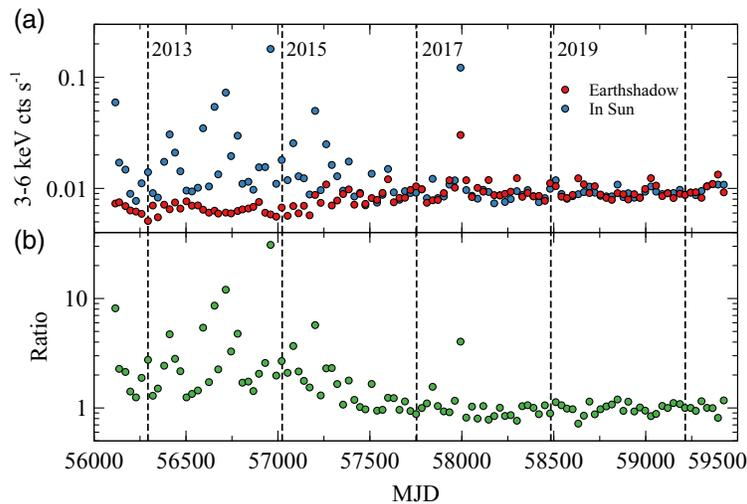
**Fig. 4** (a) A comparison of the 3 to 6 keV “In Sun” (blue) and in Earthshadow (red) count rates for the first 100 months since launch showing the excess near solar maximum in 2014 (MJD 56700) and the relative quiet during the recent solar minimum. (b) The ratio of the two rates, showing the high amount of solar activity in the first three years of the mission, as well as the enhanced activity in September 2017 (MJD 58000), during which there were multiple X- and M-class flares.
