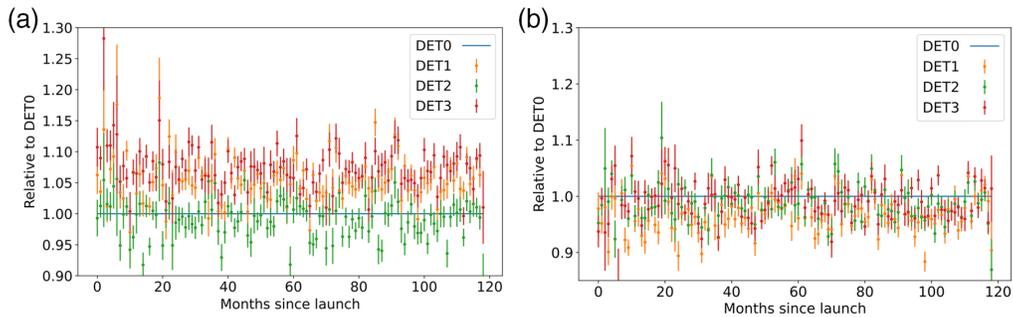
**Fig. 12** Monthly average 100 to 120 keV count rate versus time for (a) FPMA and (b) FPMB relative to DET0 on both FPMs. No clear trends with time are seen in the relative strength of the internal continuum.
