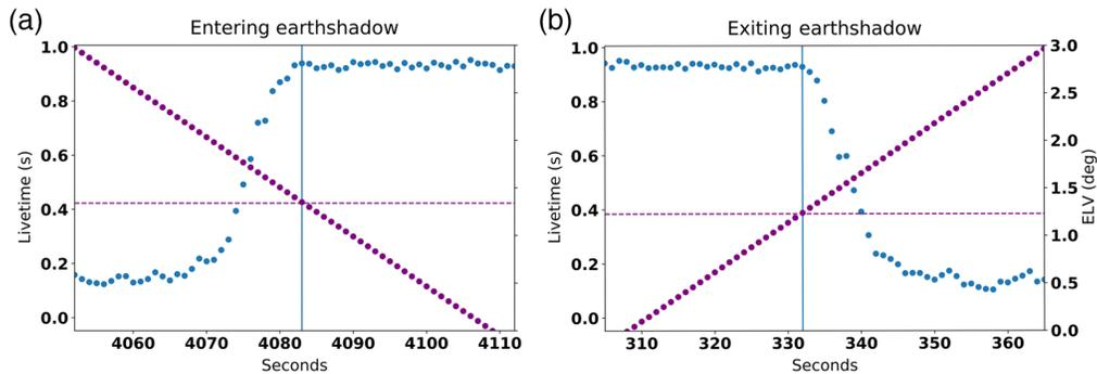
**Fig. 3** The data here show the instrument livetime (left axis, blue data points) and the ELV (right axis, purple data points) for (a) an ingress and (b) egress from Earth shadow. The vertical solid line is a by-hand estimation of when the livetime has plateaued, while the horizontal guide line shows the ELV where this occurs. This corresponds to the time when the source is 100% blocked by the Earth limb.
