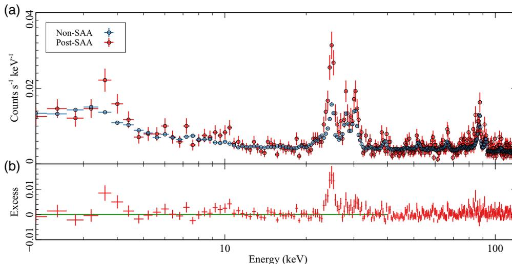
**Fig. 9** (a) Spectrum extracted just after *NuSTAR* passes through the SAA (red) compared with the non-SAA spectrum (blue). (b) The residuals between the two spectra show a clear line at  $\approx 25$  keV and a broad excess at  $\sim 3.9$  keV.
