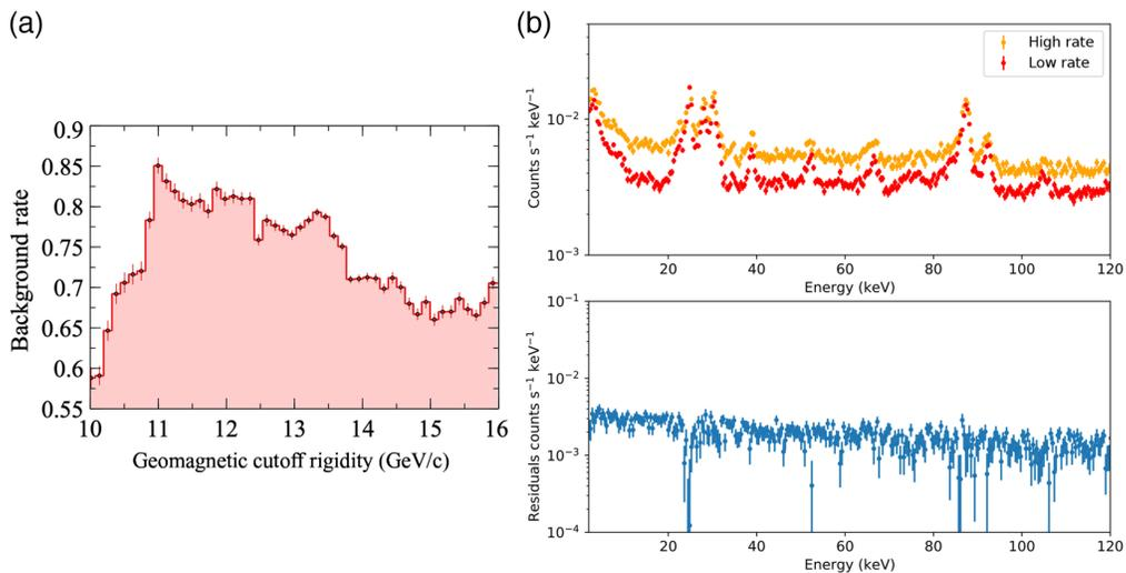
**Fig. 8** (a) Count rates distribution versus geomagnetic cutoff rigidity for April/May of 2019 showing the ridge of excess emission around 11 GeV/c and the subsequent dropoff to lower cutoff rigidity values. (b) The spectrum from “high” and “low” backgrounds (top) and the residual background showing that (outside of a deficit near  $\approx 25$  keV) the additional background is largely a featureless power-law continuum.
