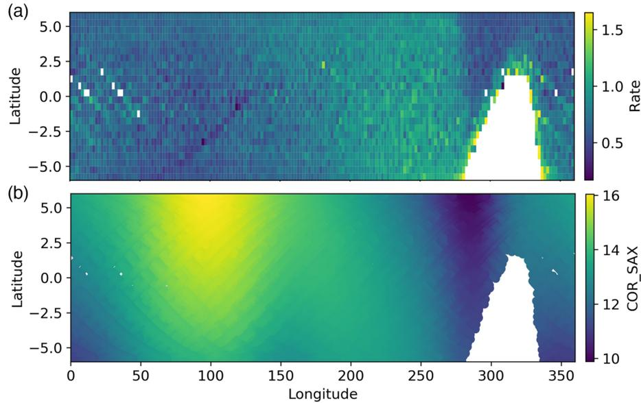
**Fig. 7** (a) The geographic distribution of the *NuSTAR* background during April/May of 2019, a “quiet” period without significant solar activity. The blank area is when the instrument is in the SAA and the instrument stops recording data. (b) The apparent east/west variations are caused by the changes in the geomagnetic cutoff rigidity.
