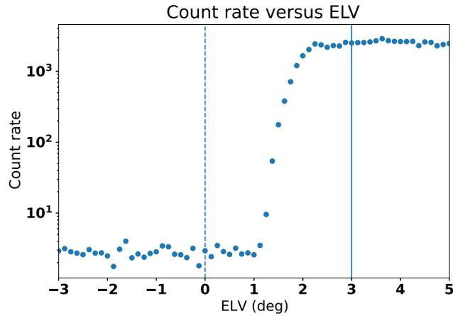
**Fig. 2** The livetime-corrected source count rate versus the angle to the Earth limb (ELV). The vertical line shows the standard cutoff for occulted science data, while the vertical dashed line shows the cutoff used in this analysis.
