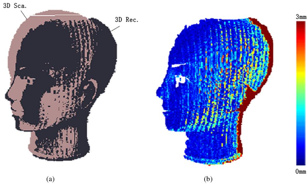
**Fig. 5** Three-dimensional (3-D) reconstruction results compared with the data from a 3-D scanner.
