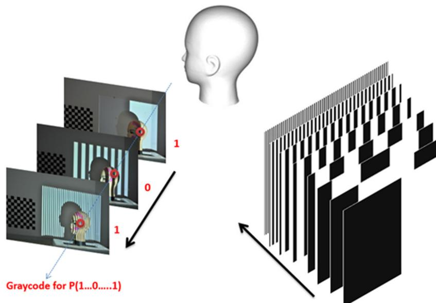
Fig. 2 Coding and decoding of the gray code.
