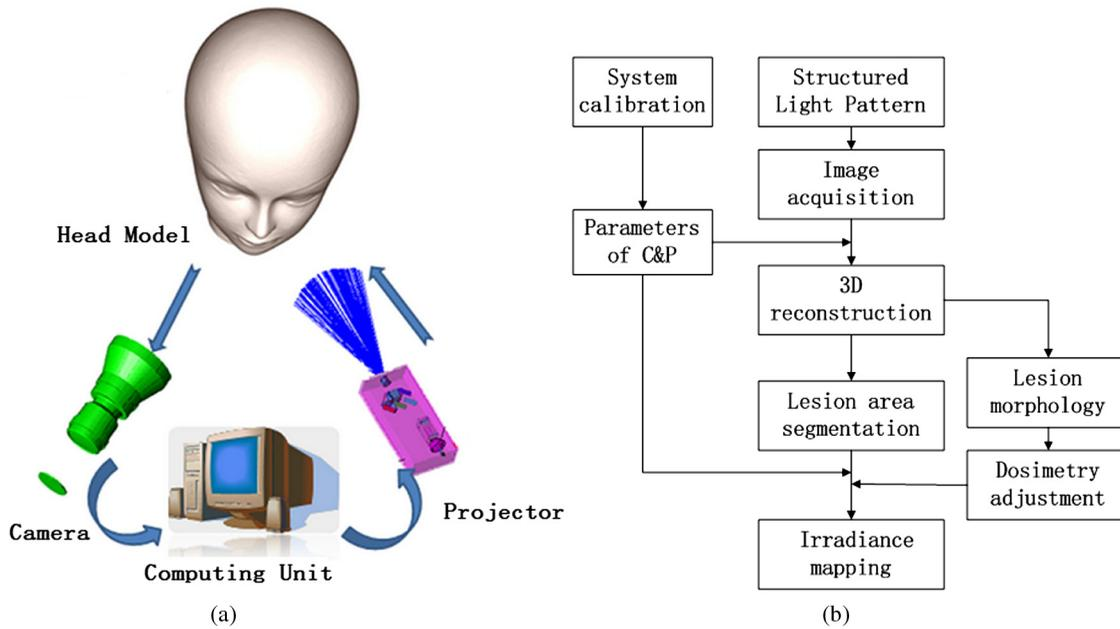
Fig. 1 (a) System configuration and (b) the software flow chart.
