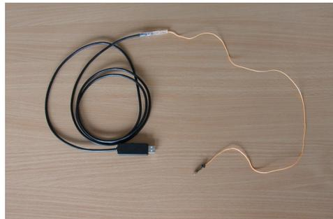
**Fig. 3** Finished USB endoscope allowing retrograde scanning of the upper part of the digestive tube.
