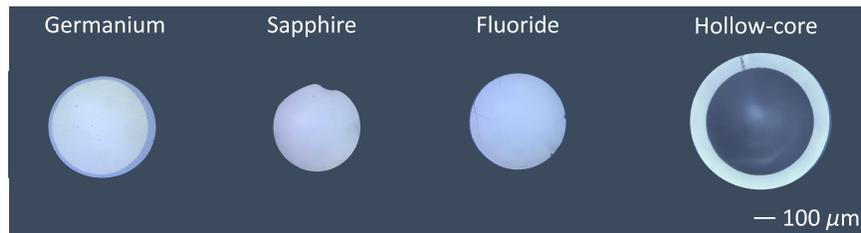
**Fig. 1** Microscopic images of the fibers' polished surfaces.
