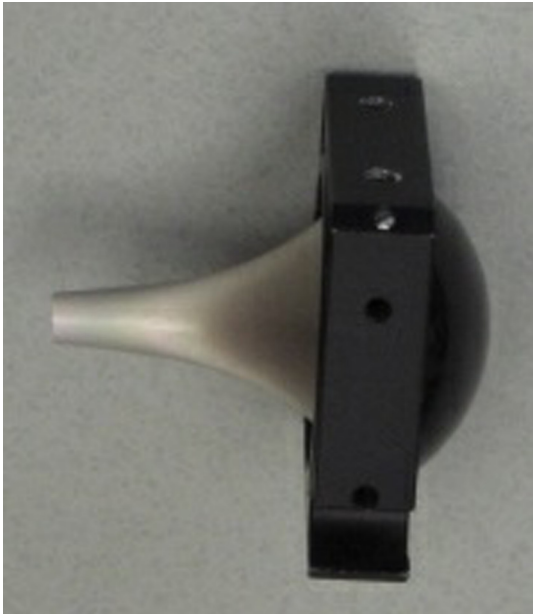
Fig. 1 Dragonfly optic (prototype #2) mounted in a 40 mm square frame.
