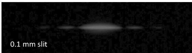
Fig. 6 Photo of observed diffraction pattern for a He–Ne laser through a 0.1-mm vertical slit. Photon scattering is perpendicular to the slit. (Credit: Jordgette 2010.)
