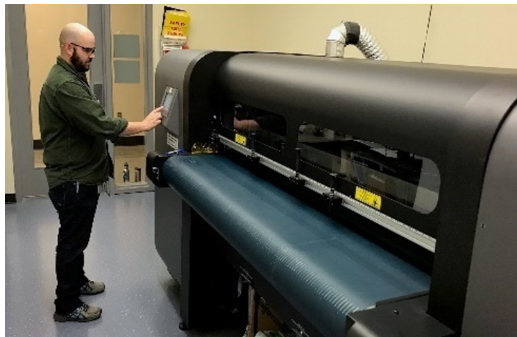
Fig. 7 Customized one-meter format graphics inkjet printer used to produce freeform GRIN optics.
