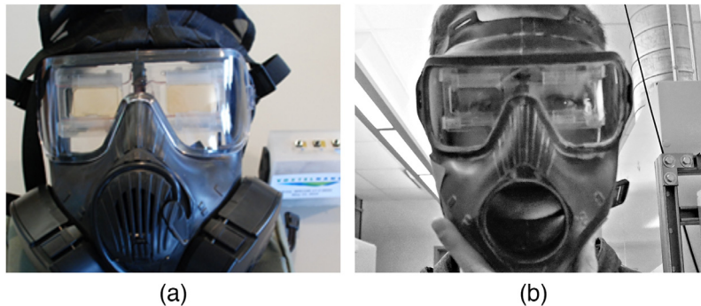
Fig. 9 Picture showing VCI in a respiratory mask (a) inserted in Avon50 mask and (b) worn by user (with filter removed).
