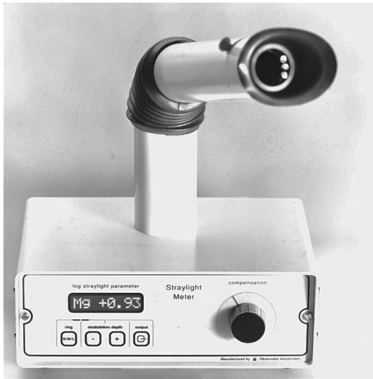
Fig. 1 Entoptic straylight at 3.5, 10, and 28 deg can be determined with the straylight meter depicted in this photograph, employing the direct compensation method.
