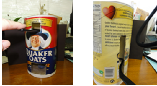
Figure 2. Image of “microscope” made using magnifying lenses and oatmeal containers – based on the design in Van Cleave, 1993 14
