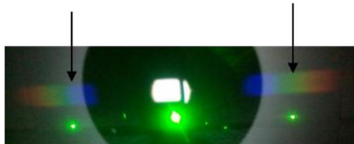
Figure 10. Comparison of the white light scatter with the diffraction pattern of the green marker.
