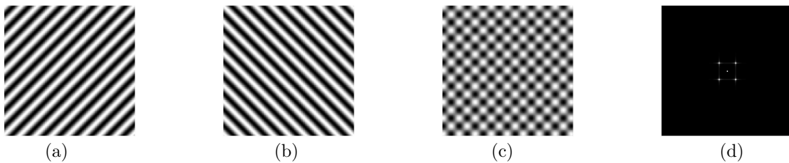
Figure 2. Image of (a) first grating; (b) second grating; (c) addition of (a) and (b); (d) |\mathcal{FT}| of (c).
