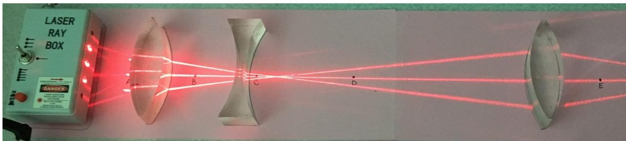
Figure 1. Laser ray box with converging and diverging lenses. Here points A, B, C, D, and E represent points where students could identify parallel, converging, or diverging rays and wavefronts, positive, negative, or zero vergence, and real, virtual or distant objects and images for each lens.
