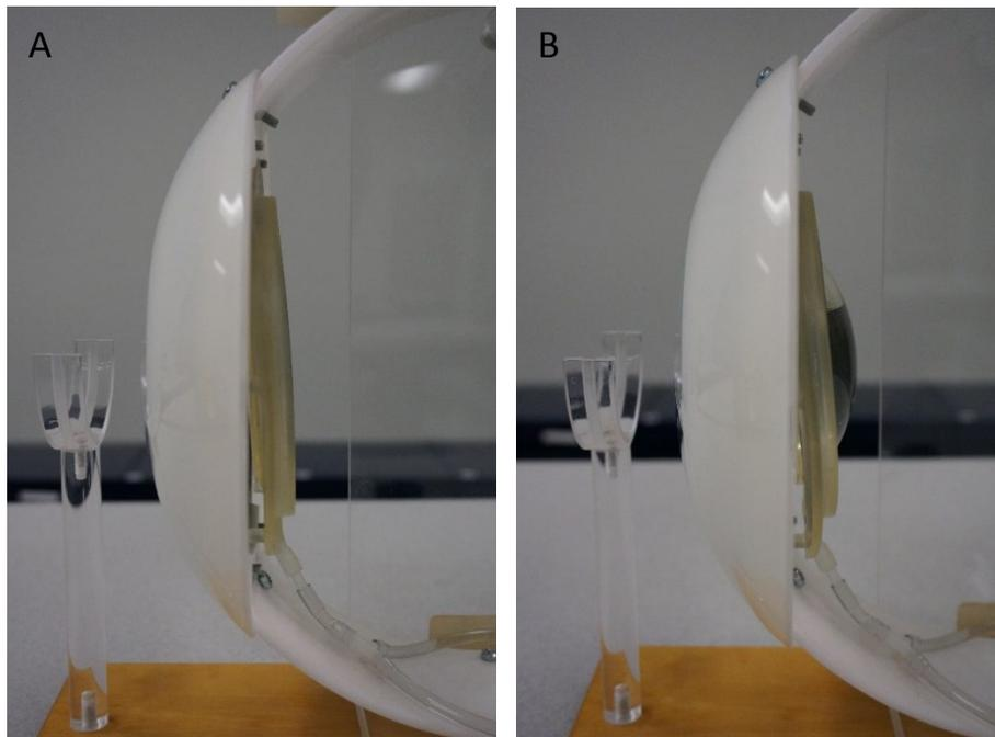
Figure 3. Close-up images of the adjustable lens from the model eye discussed in figure 2. The adjustable diaphragm is shown on the left with no water and on the right filled with water. The increase in radius of curvature and increase in power can be used to demonstrate ophthalmic concepts including myopic and hyperopic eyes and accommodation.
