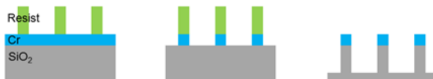
Figure 3. Manufacturing process of binary surface relief gratings by e-beam lithography (left image) and reactive ion etching of the chromium layer (middle image) and SiO 2 (right image).
