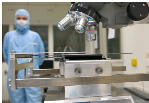
Figure 9. Setup for verification whether the grating lines and the triangular prism surfaces are perpendicular. The bonded wafer is on top of the dark prism. The excess wafer parts are not yet removed. Above and below the wafer are aluminum plates with parallel edges. A spring pushes the lower alignment plate against the prism side. The rotation is determined from the distances between the upper aluminum plate edge and the alignment marks on the bonded wafer.
