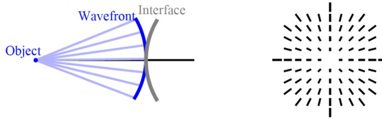
**Figure 4** (Left) The spherical wavefront from an on-axis object point incident on a spherical interface has an angle of incidence of zero at the center of the beam. (Right) The paraxial angle of incidence for an on-axis wavefront at a spherical surface increases linearly from the center and equals the marginal ray angle of incidence at the edge. Line lengths indicate the angle of incidence and the orientation indicates the plane of incidence.
