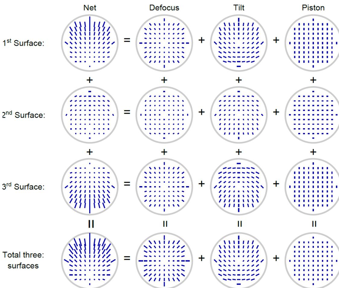
**Figure 10** The polarization contribution from three surfaces is shown in the left column. Each of these polarization aberration maps can be decomposed into the summation of a defocus term (second column), a tilt term (third column) and a piston term (right column). These defocus, tilt, and piston columns can also be summed separately, by adding columns, to equal the bottom row’s defocus, tilt, and piston terms, which sum to the overall polarization aberration map (lower left).
