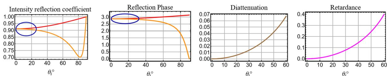
**Figure 1** (Left) Fresnel intensity reflection coefficients for Aluminum, 800 nm: red s-polarized, orange p-polarized. (Second) Phase change on reflection in radians. The blue circles highlight the regions of quadratic behavior near normal incidence. (Third) Corresponding diattenuation, degree of polarization when unpolarized light is incident. (Right) Retardance in radians.
