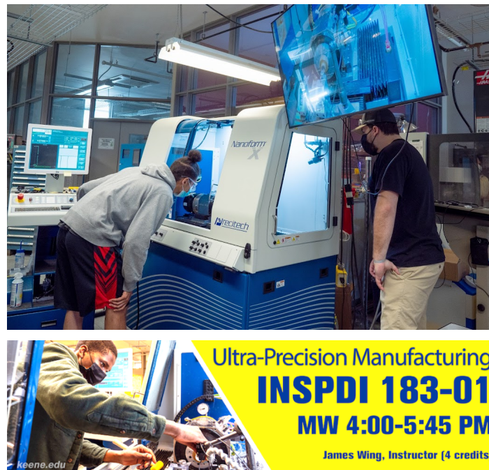
Figure 3: Students get hands-on experience on the Nanoform X Precitech lathe as part of the INSPDI 183 course
