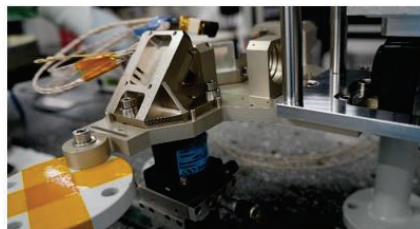
Figure 4. Configuration with the corner cube
