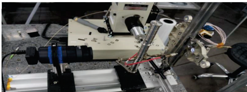
Figure 6. Mounting for beam centering adjustment
