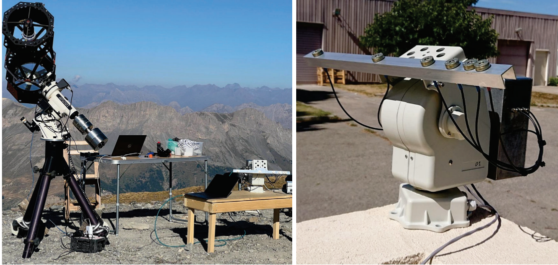
Figure 6: (Left) SHABAR prototype at dawn by Saint-Véran observatory site, 3000 m high. (Right) Close-up view of the SHABAR prototype, installed on our office roof. All instrumentation is embedded in the rear water-tight enclosure.
