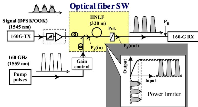
Fig. 8 Amplitude noise suppression using nonlinear fiber<sup>21</sup>
