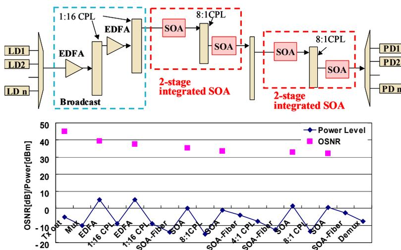
Fig.5 Multi-gate SOA switch architecture for Peta-flops ultra-high performance computer system<sup>12</sup>.
