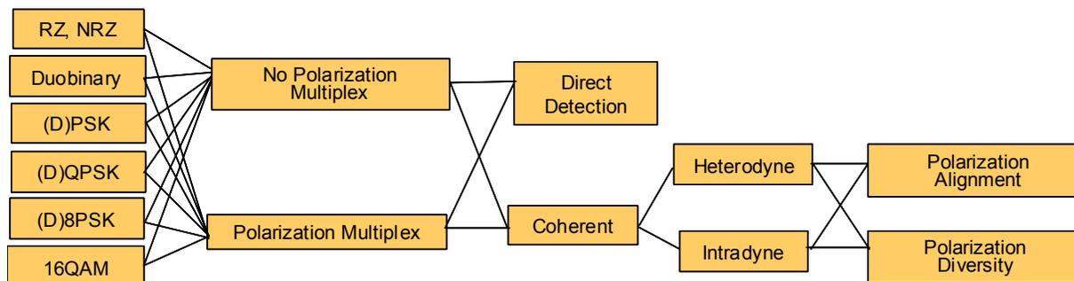
Fig. 3 Transceiver technology options
