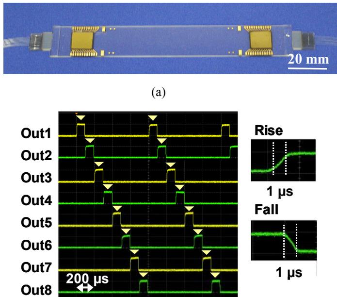
Fig.4 High-speed switch; (a) outer view, and (b) its optical switching response<sup>11</sup>
