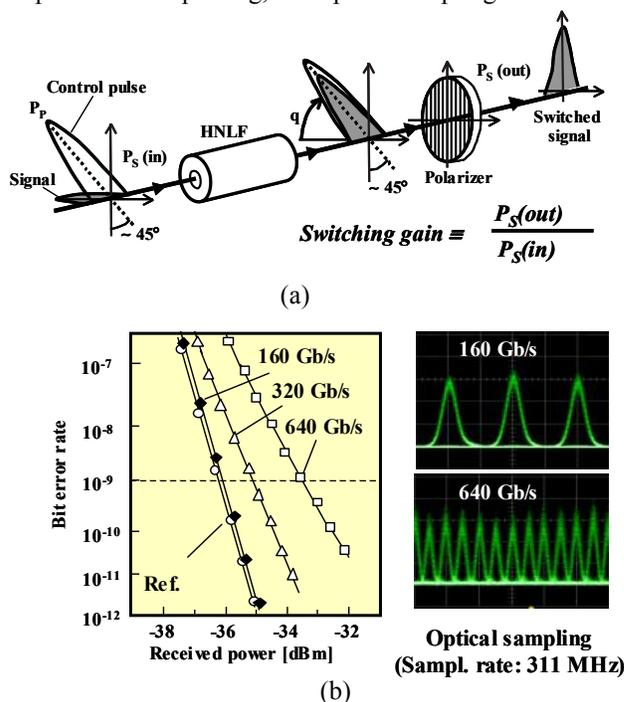
Fig. 9 Optically parametric amplified fiber switch. (a) Switching configuration, (b) BER and sampling waveform
