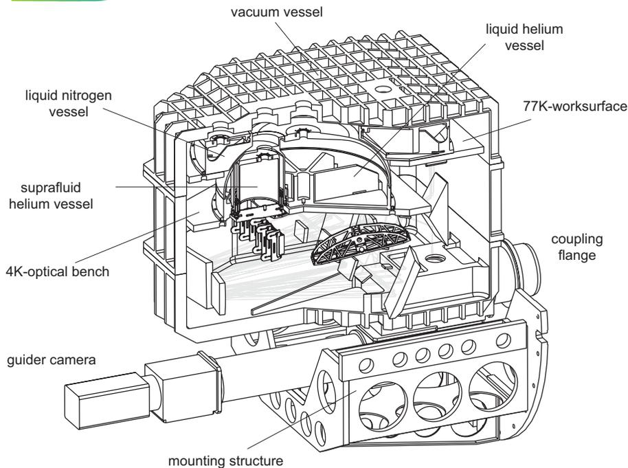
Figure 1. A cut through the *FIFILS* cryostat. The optical components are mounted on the work surfaces attached to the cryogen vessels. Light from the SOFIA telescope is entering the instrument from the right via the coupling flange.
