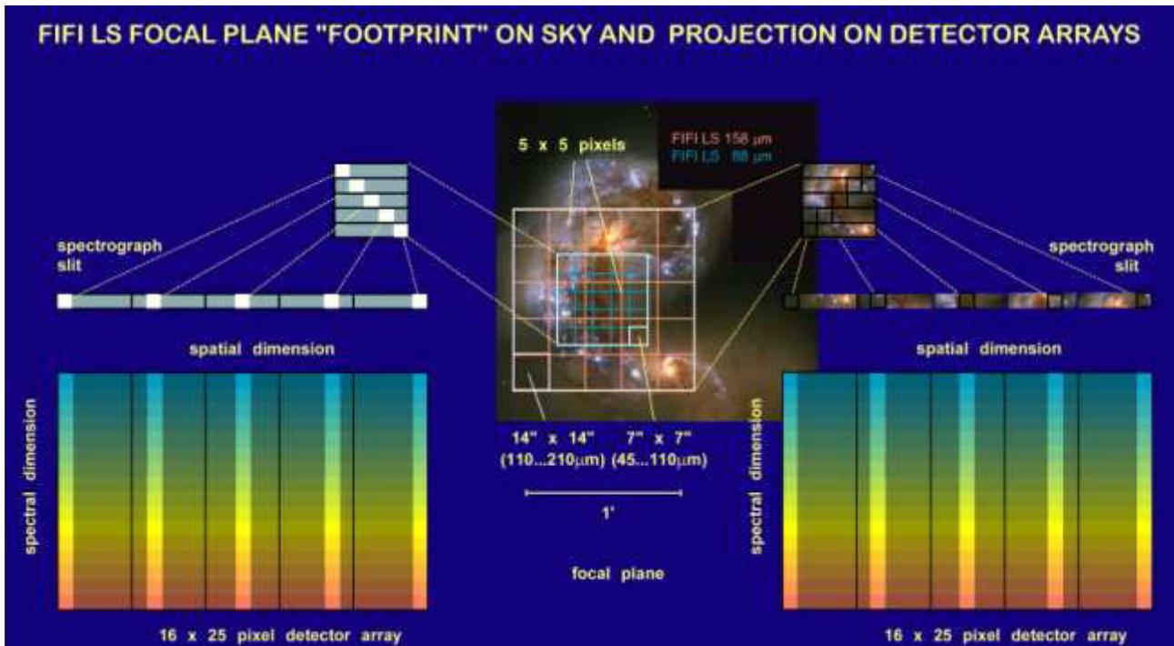
Figure 2. Field-of-view and image slicer concept: The field-of-view, which can e.g. contain the antennae galaxy, consist of 5x5 spatial pixels for each spectral channel. Both channels observe the same area, but at different pixel scales. The image slicer dissects the FOV into 5 slices which get rearranged along the slit of the spectrometer to then get dispersed onto 16 pixels. The result is a 25 spectra each 16 pixels wide or a  $5 \times 5 \times 16$  data cube.
