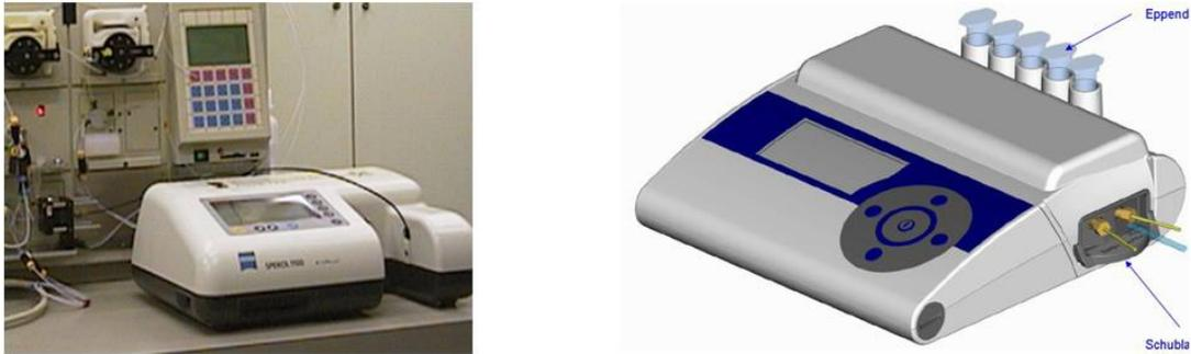
Figure 7. Instrumentation for spectral RfS (left) and commercialized single wavelength set-up (Biometrics)<sup>18</sup> (right)
