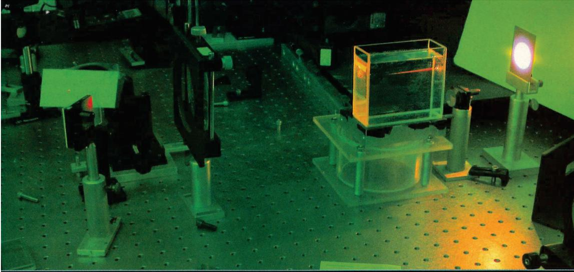
EXPERIMENTAL SETUP to produce supercontinuum light sends high-intensity laser light (red) through a suitable optical medium (here a container of liquid) that greatly broadens the light's bandwidth (white light).
