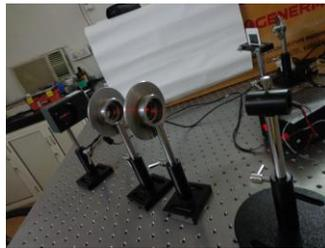
Fig.8: Polarisation setup for Malus law
