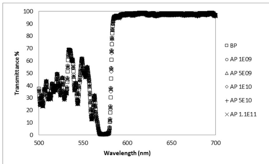
**Fig. 7.** Transmittance of a Dichroic filter before and after proton radiation according to the different accumulated fluence\* ( $p^+/cm^2$ )
