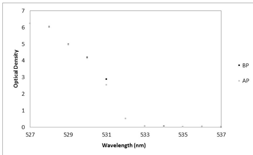
Fig. 12. Optical Density of a Long Pass filter before and one week after  $1.1E11 p^+/cm^2$  accumulated proton fluence\*
