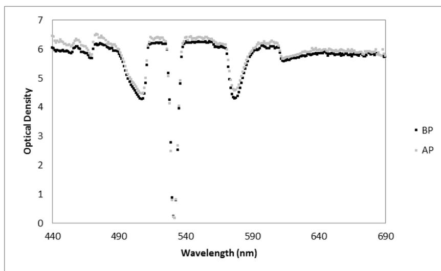
Fig. 11. Optical Density of LL01-1 before and one week after  $1.1E11 p^+/cm^2$  accumulated proton fluence \*
