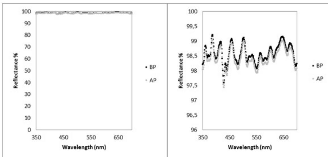
Fig. 9. Reflectance of a mirror before and one week after  $1.1E11p^+/cm^2$  accumulated proton fluence \*
