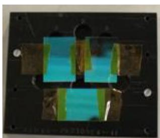
Fig. 5. Distribution of the Dichroic filters on the TSH.
