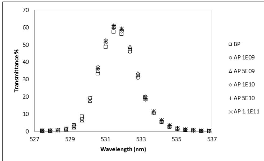
**Fig. 6.** Transmittance of a Laser Line filter before and after proton radiation according to the different accumulated fluence\* ( $p^+/cm^2$ )
