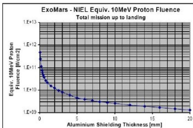
Fig. 3. Equivalent 10 MeV total mission protons fluence up to landing vs Al shielding
