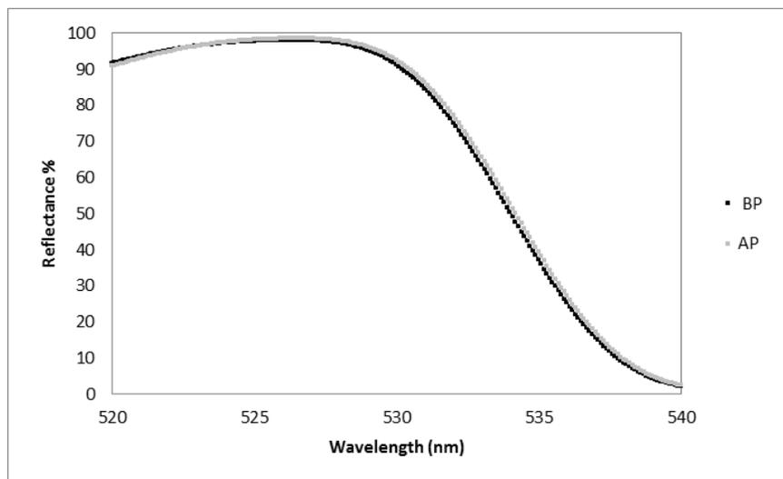
Fig. 10. Reflectance of a Dichroic filter before and one week after  $1.1E11 p^+/cm^2$  accumulated proton fluence \*
