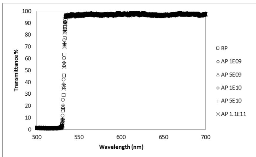
Fig. 8. Transmittance of a Long Pass filter before and after proton radiation according to the different accumulated fluence\* ( $p^+/cm^2$ )
