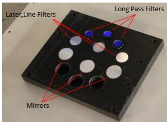
Fig. 4. Distribution of the Laser line filters, Long Pass filters and mirrors on the TSH.
