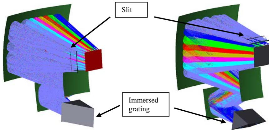
Figure 2 Layout of two IG based designs. On the left the slit and the detector are next to each other on the right they are in the plane of the TMA mirrors.
