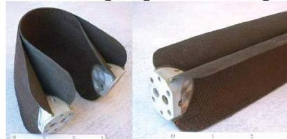
Fig. 8. EMC actuator example in the stowed and deployed configuration.
