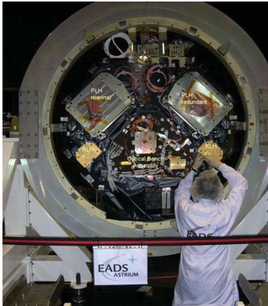
Fig. 7. ALADIN structure with laser heads and receiver during integration of the test model
