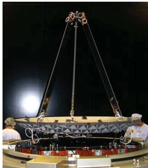
Fig. 6. ALADIN telescope test model during integration
